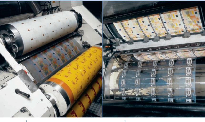
Plate cylinders for printing  $\leqslant$ 50 banknotes and a rubber printing blanket in an offset printing machine.
