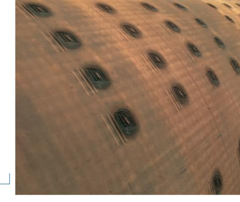
Cylinder mould for the production of €5 banknote paper, showing the embossed images for the watermarks.
