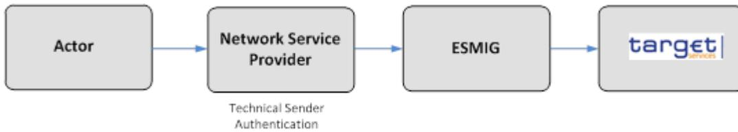
In case of successful authentication of the technical sender, the TARGET Services, common components or applications get the certificate DN of the technical sender. The TARGET Services, specific/common components or applications may use this certificate DN later on, during the authorisation process.
