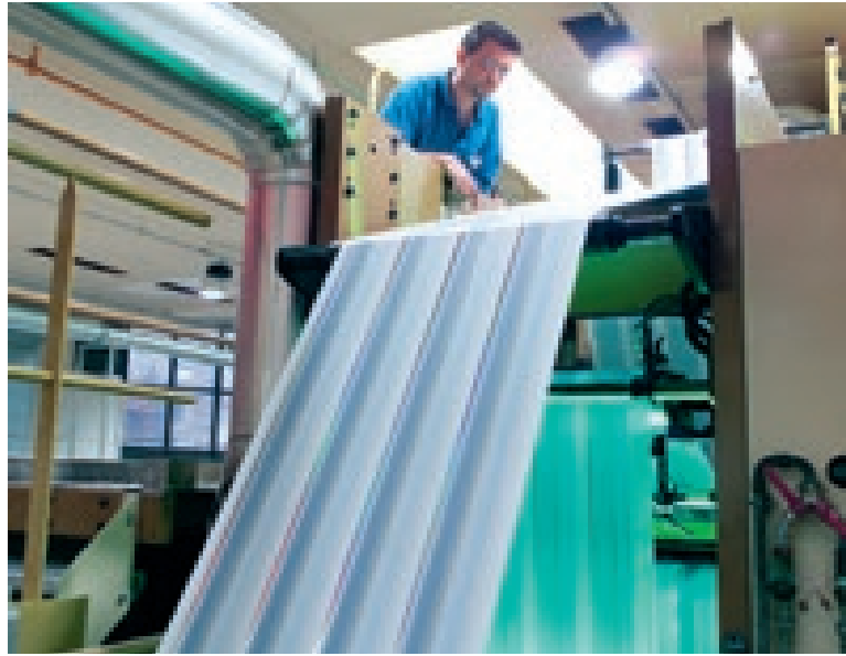
◆ Fig. 35 Different printing works produced euro banknotes by different methods, which made uniform quality an even greater challenge. The printing works of the Banque de France used sheet printing but also web presses, where the banknote paper is fed into the printing machine from a large roll and the different stages of printing are implemented one after another on the same machine. Only at the final stage are the banknotes cut into sheets. ◆
