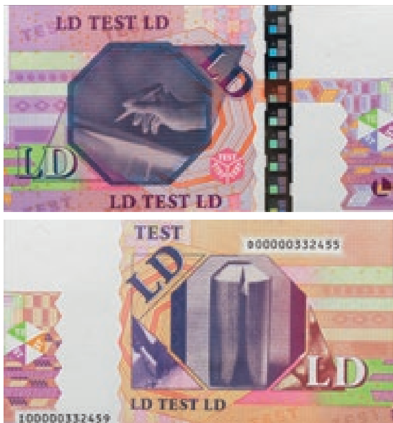
◆ Figs. 60 Sample notes were produced for laboratory testing, using various materials and coatings that were potentially suitable for low-denomination banknotes. ◆
