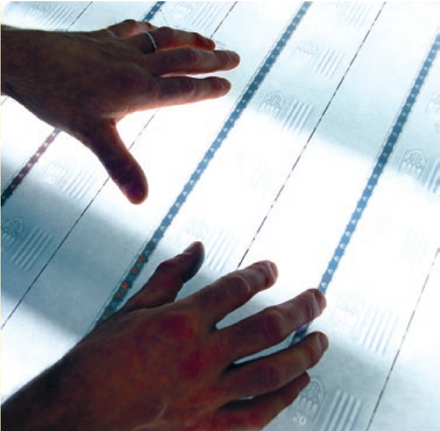
◆ ————— ◆ Fig. 36 Ready banknote paper being inspected at a paper mill of the Banque de France. Security threads, like watermarks and hologram stripes, are incorporated into banknotes at the paper mill.
